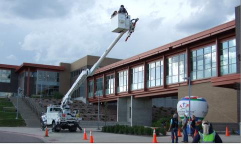
Above: At the 74th annual meeting of members of Mountain View Electric Association, MVEA linemen offered co-op members rides in the bucket truck used for line maintenance on overhead "energized" lines. The bucket is 55 feet high when fully extended and is strong enough to lift electric lines that weigh about one pound for every foot of line, said Claud Hugley, Operations manager, who is retiring this year after 42 years of service. Photo by Lisa Hatfield
