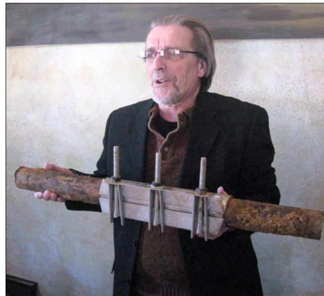
Above: Palmer Lake Water Trustee Michael Maddox displays the sample of an approximately 70-year-old galvanized steel water pipe section he showed at the Palmer Lake Town Council meeting on Dec. 6. The pipe is typical of the water lines needing to be replaced in Palmer Lake, with calcification narrowing the diameter of the pipe and multiple leaks requiring metal patches to keep drinking water from seeping into the ground. Photo by Lisa Hatfield.
